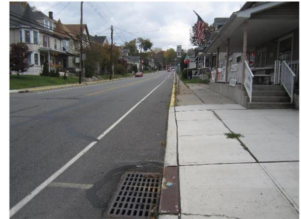
Parking spots to the south of the building can be replaced with porous asphalt to capture and infiltrate stormwater. A stormwater planter can be built into the sidewalk in front of the building to intercept stormwater runoff from the roadway and sidewalk. A preliminary soil assessment suggests that more soil testing would be required before determining the soil's suitability for green infrastructure.
